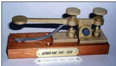
Figure 2: Telegraph equipment to send electrical signal
